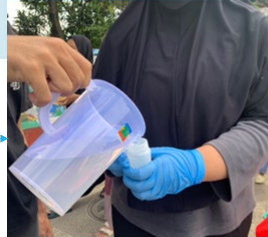
Put wastewater sample into plastic & glass bottles
