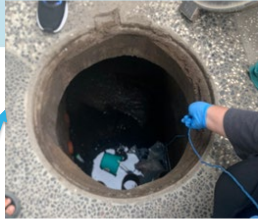
Take wastewater samples using a bucket
